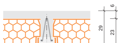
strop Porotherm 23/50/6 strop Porotherm 23/62.5/6
