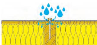
Installation of counter battens without sealing.
