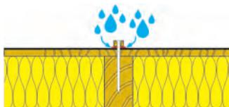
Installation of counter battens with sealing -moisture does not penetrate.
